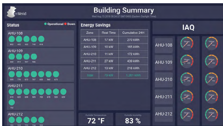
The enVerid Cloud enables users to monitor and manage HLR modules and building IAQ
